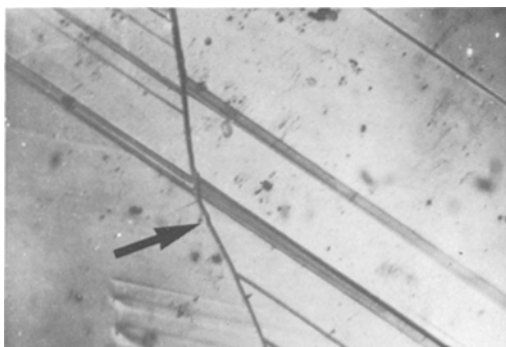
Figure 3 Single crystal with a \langle 110 \rangle compression axis. The face shown is the \{111\} face, with glide lines corresponding to \{100\} glide planes. The arrow indicates a crack.
